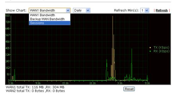
The horizontal axis represents time. Yet the vertical axis has different meanings. For WAN1 Bandwidth chart, the numbers displayed on vertical axis represent the numbers of the transmitted and received packets in the past.
