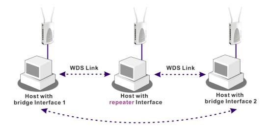
The major difference between these two modes is that: while in **Repeater** mode, the packets received from one peer AP can be repeated to another peer AP through WDS links. Yet in **Bridge** mode, packets received from a WDS link will only be forwarded to local wired or wireless hosts. In other words, only Repeater mode can do WDS-to-WDS packet forwarding.
