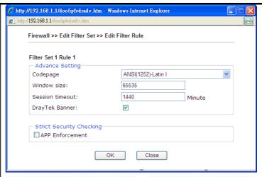
Codepage - This function is used to compare the characters among different languages. Choose correct codepage can help the system obtaining correct ASCII after decoding data from URL and enhance the correctness of URL Content Filter. The default value for this setting is ANSI 1252 Latin I. If you do not choose any codepage, no decoding job of URL will be processed. Please use the drop-down list to choose a codepage.
