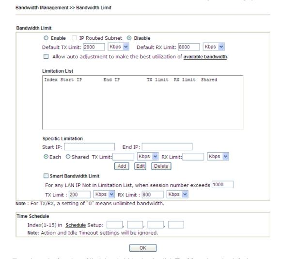
To activate the function of limit bandwidth, simply click **Enable** and set the default upstream and downstream limit.
