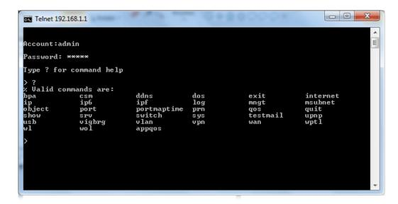
For users using previous Windows system (e.g., 2000/XP), simply click **Start** >> **Run** and type **Telnet 192.168.1.1** in the Open box as below. Next, type admin/admin for Account/Password. And, type ? to get a list of valid/common commands
